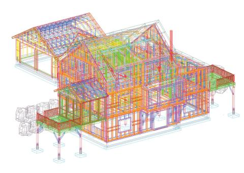
Using state-of-the-art 3D software, we first build each home virtually to provide our clients with a clear understanding of the design, and identify potential issues before construction begins. Our fabrication process starts with computer-controlled machinery in our shop, and culminates in the rapid assembly of precision-built components on site.
