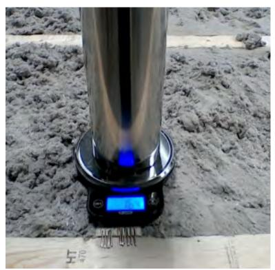
In addition to checking the insulation visually and by "feel," we periodically confirm the density by weighing core samples taken from insulated panels. A density of 3.5 to 4.0 pounds per cubic foot provides excellent insulation and prevents settling.
