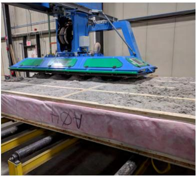
Once the cellulose has been "dense packed" into the wall and roof panels, we install a continuous exterior layer of insulating sheathing made from a different form of cellulosewood fiberboard—to secure the insulation in place. For roof panels, we may install the finished roof surface such as sheetrock or boards, and for wall panels, we install windows and doors into the panels before carefully bundling and shrinkwrapping the panels for shipping to site.
