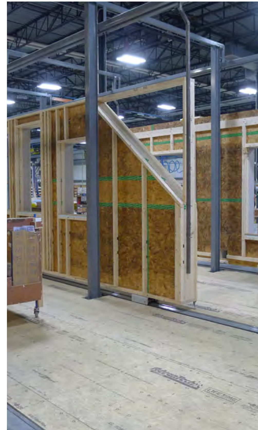
Wall panels in gantries (interior side)
