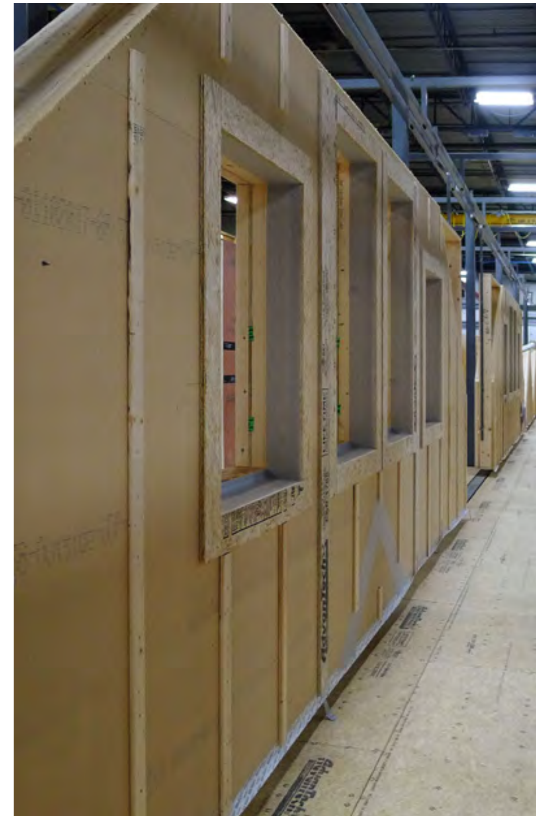
Wall panels (exterior side)
