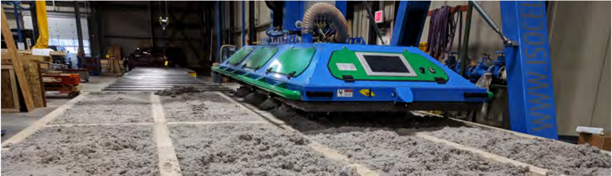
Installing cellulose in roof panel
