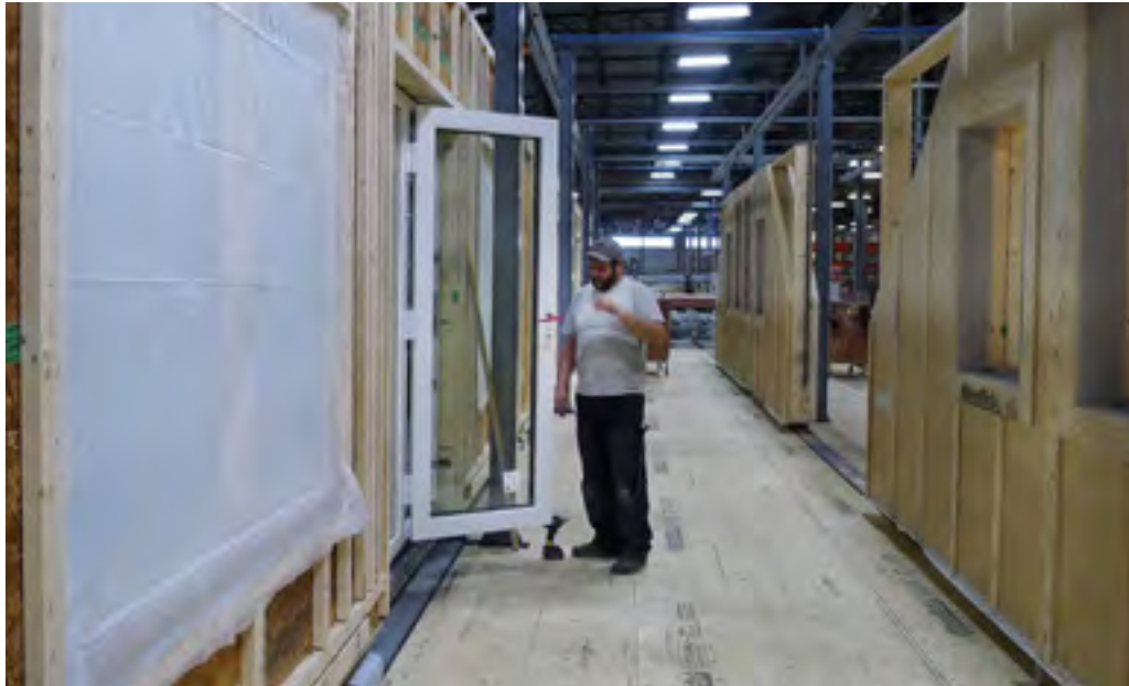
Door installation in wall panel
