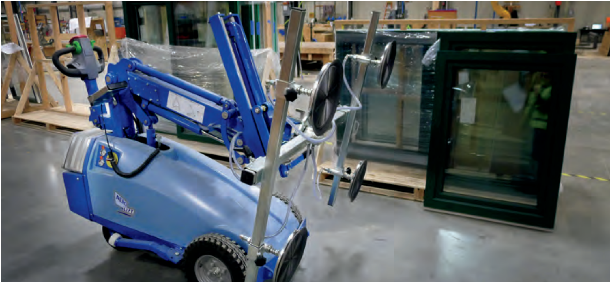
Window/door installation-assisting "robot"
