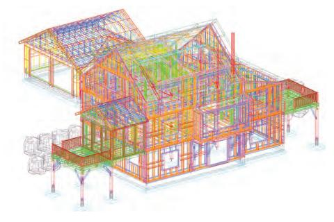
By using state-of-the-art 3D software to first "build" each home virtually, we are able to provide our clients with a clear understanding of the design, and identify potential issues before construction begins. Our fabrication process starts with computer-controlled machinery in our shop, and culminates in the rapid assembly of precision-built components on site.
