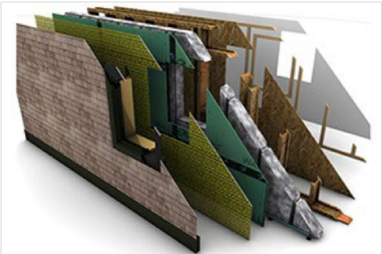
A cross-section of Unity's OBPlus Wall System wall panel, featuring moisture barriers, cellulose fill, and service layer.
